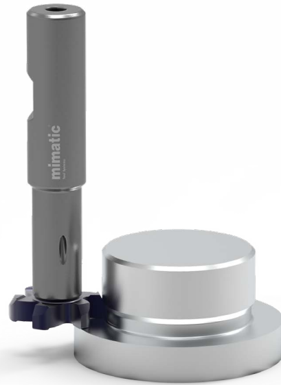
Milling a thread undercut according to DIN 76
