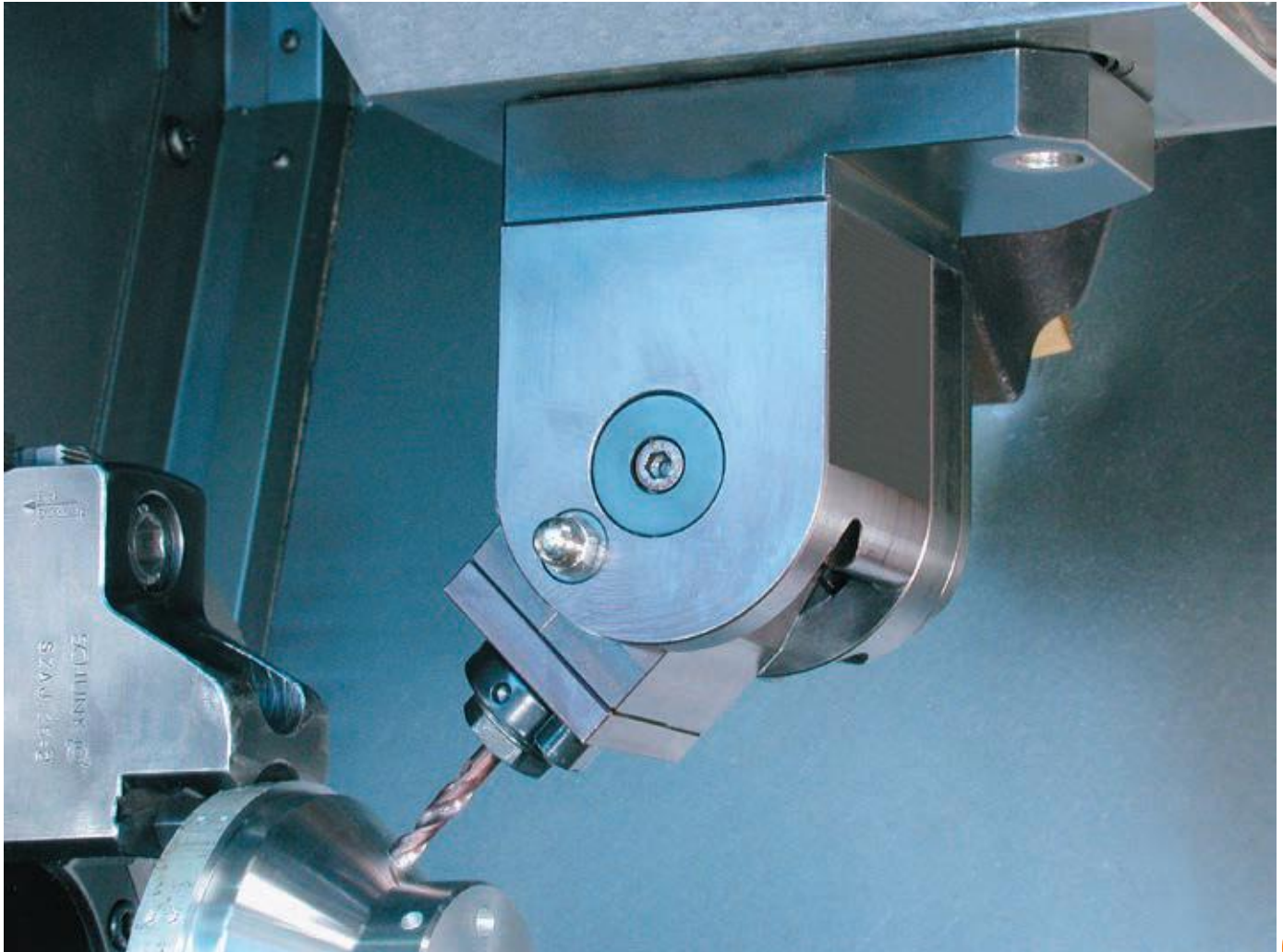
Picture shows an adjustable angle head (90°) on a Mazak SQT 18 MS drilling holes on 45°.
